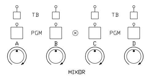
The 4 audio inputs can be switched to either the PGM or TB mix. This is done by pressing the red or white push buttons on the top panel. These switches as well as routing the audio also turn the channels input on/off. A LED next to the push button indicates when a channel is on and routed.
